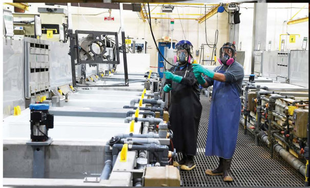
Electroplaters Adrian Alvarado and Thomas Barrera conduct the first component immersion.
