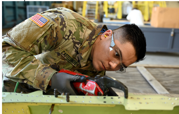
Above: An unidentified soldier from the 12th Combat Aviation Brigade, gains valuable on-the-job experience by working on the rivets of a helicopter skin during dissassembly at CCAD. Photo by Ervey Martinez.
